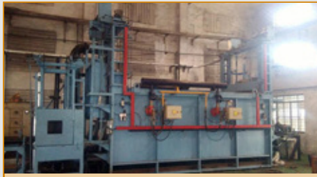
Continuous Ht Furnace
